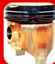
Neglected Engine Oil System - deposit build up around piston & rings reducing efficiency.
