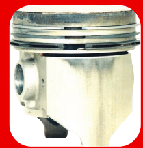
Well maintained Engine Oil System - rings free to move improving compression.
