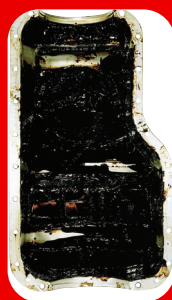
Dirty neglected Engine Oil System.
