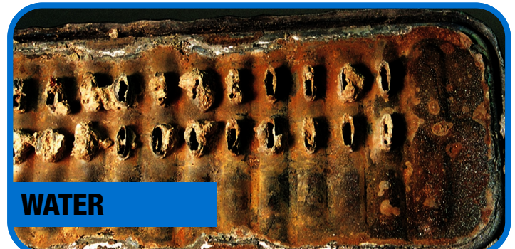
Radiator using coolant vs radiator using water
