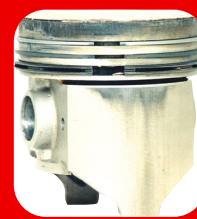
Well maintained Engine Oil System - rings free to move improving compression.
