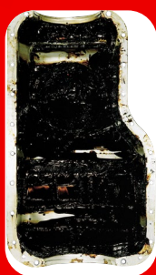
Dirty neglected Engine Oil System.
